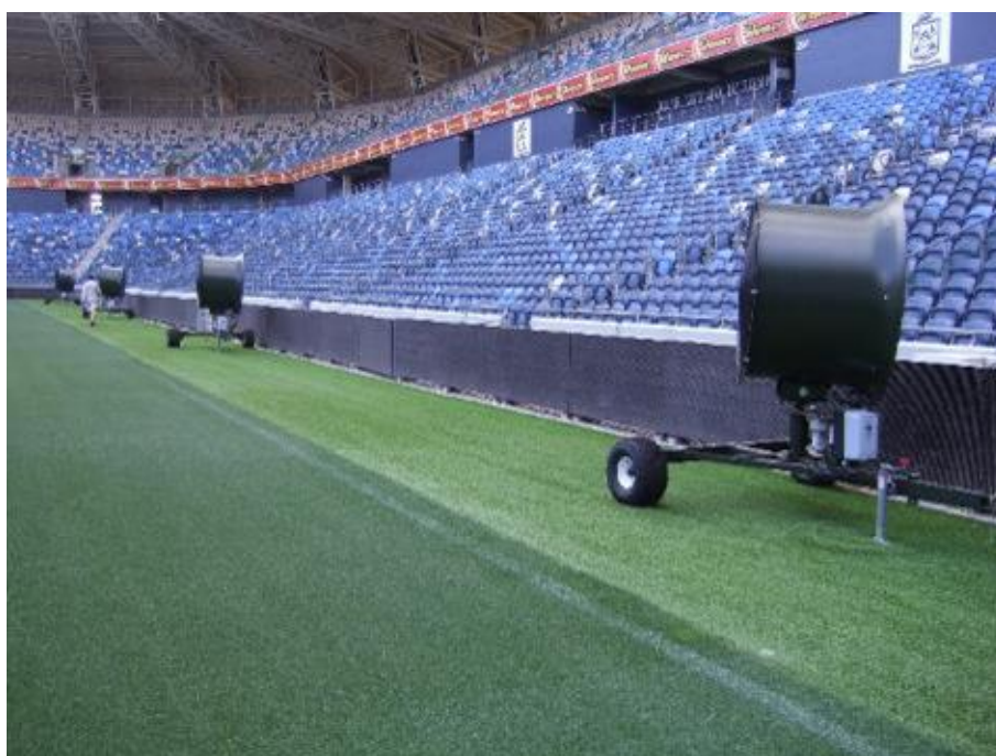
Fig. 8. Proprietary pitch-side turf fans used to enhance air flow across a pitch. A full-size rugby pitch will require a minimum of 10 units.
