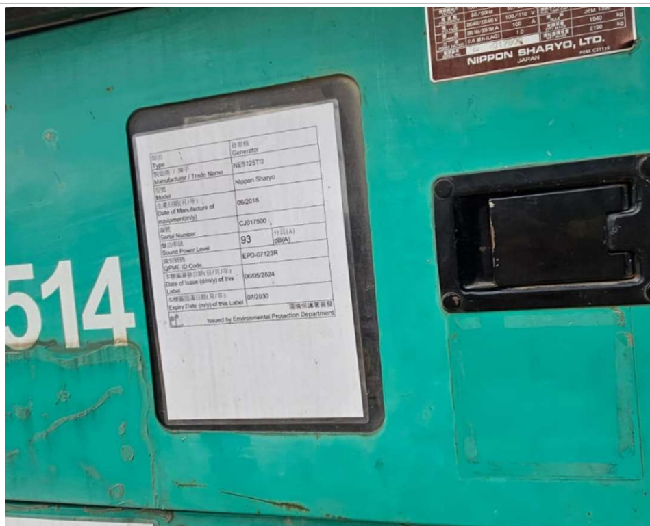
Photo 2: Power Mechanical Equipment with Quality Power Mechanical Equipment (QPME) labels were used at site to lower the noise nuisance to the nearby residents.
